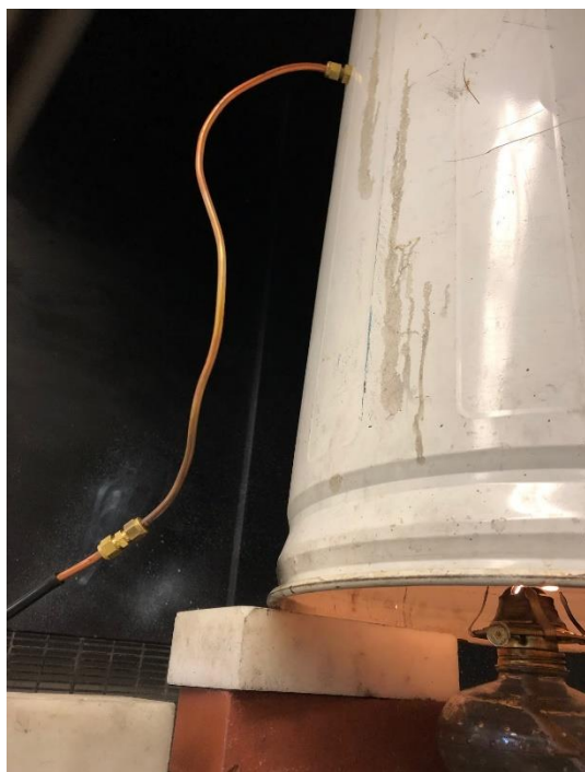
Figure 12. Kerosene lamp lit beneath a bucket where smoke can accumulate. PA660 sample inlet will be connected to the bucket so that smoke can be drawn through the instrument
