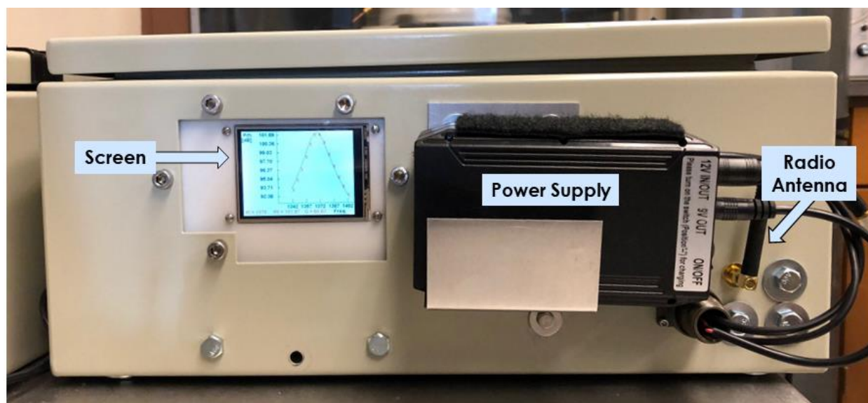
Figure 2. Photograph of the side of the PA660 enclosure with its main components labeled.
