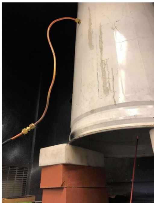
Figure 10. Incense stick lit beneath a bucket where smoke can accumulate. PA660 sample inlet will be connected to the bucket so that smoke can be drawn through the instrument.
